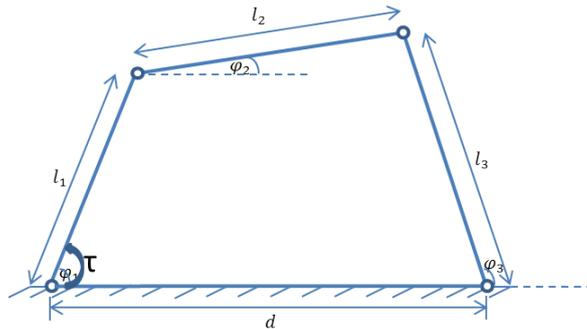
Fig. 1: Four-bar linkage
