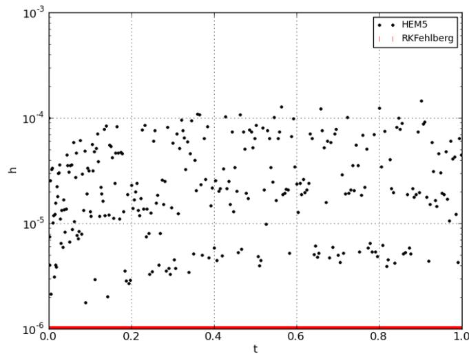
Fig. 4: Four-bar linkage. Evolution of the time step with the simulation time.
