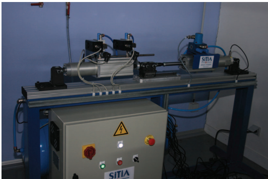
Fig. 1: [10] the electropneumatic system - On the left hand side is the “main” actuator whose its position is controlled. On the right hand side is the “perturbation” actuator whose load force is controlled.
