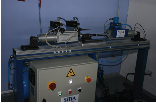
Figure 1: [18] Left. Photo of the electropneumatic system - On the left hand side is the “main” actuator whose its position is controlled. On the right hand side is the “perturbation” actuator whose the load force is controlled. Right. Scheme of the electropneumatic system - This figure displays the mechanical and software structures. The software structure is based on a dSpace board on which the position controller of the “main” actuator is implemented. The mechanical structure is composed by two actuators, the “main” one (left hand side) and the “perturbation” one (right hand side).
