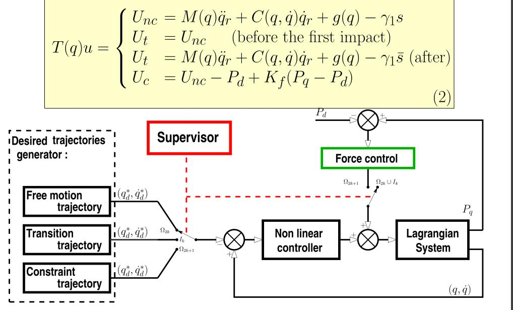
The supervisor switchs between the different trajectories according to this graph:
