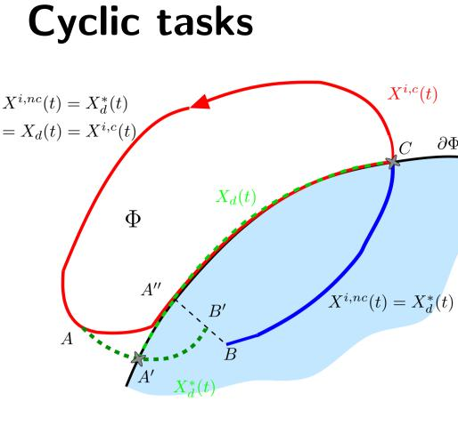
The desired trajectory CAA'B'BCtends to penetrate the surface for imposing stabilisation on  $\partial \Phi$ . But  $\partial \Phi$  if the desired trajectory always violate the constraint then the impacts occur always and the tracking can not be asymptotically stable. The strategy is to use a desired trajectory which evolve during the cycle. The curve AA'B is adapted in function of the tracking error. It will tend to the
