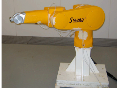
Figure 7: Flat configuration of a Stäubli Rx90
